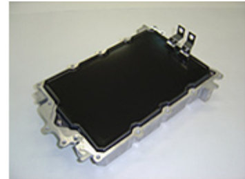
HV inverter smoothing film capacitors
