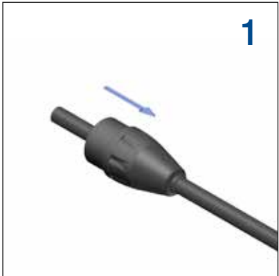
Slide the nut (Backshell) onto the cable
