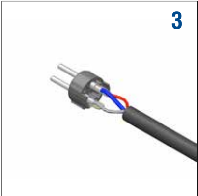
Solder the wires to the contacts.
