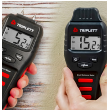
MS150 (Pin and Pinless) – Measures moisture content in wood (5 to 50%) and other building materials (1.5 to 33%). Pinless measurement (6 to 99.9%) for non-invasive testing.
