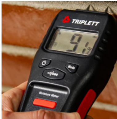
MS100 (Pin Only) – Pin Moisture Meter measures moisture content in wood and other building materials (1.5 TO 50%)
