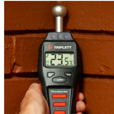
MS300 (Pinless Only – Spherical Ball Style) Measures moisture content in wood and other building materials (0.1 to 99.9%). Spherical design to get into wall and ceiling corners. Measures down to 4" depth.
