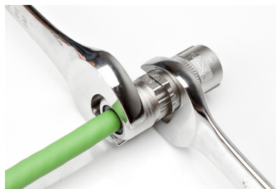
Step 16 - Tighten to 5-7 N/M using 25mm wrench
