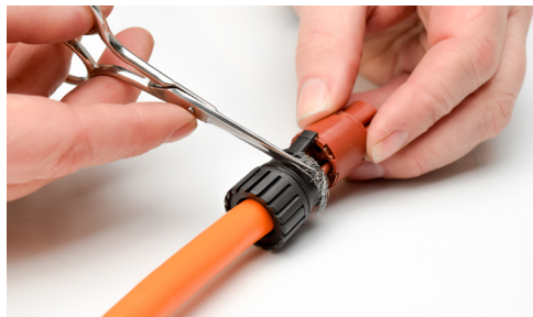
Step 14 - Trim shield as shown
