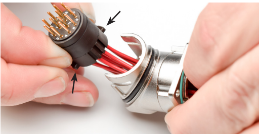
Step 5 - Locate keys on sides of insert
