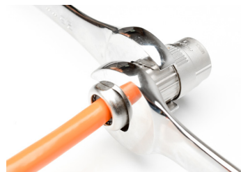
Step 17 - Tighten to 5-7 N/M using 25mm wrench
